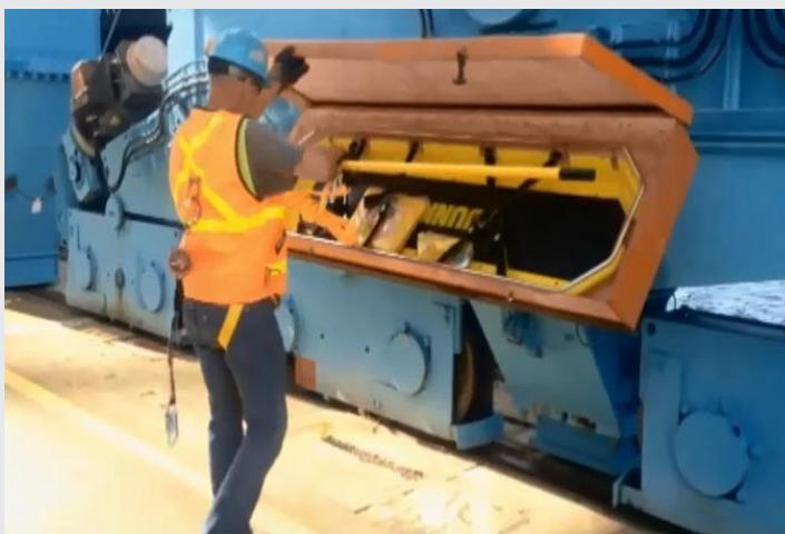
3. Be properly locked in with aloft gear to perform rescue and Connect Large Hook to corner of Crane Spreader Bar.
